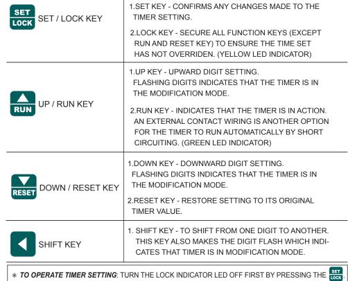
ONCE THE LOCK INDICATOR IS OFF, PRESS TO MAKE DIGITS FLASHING. THIS PREPARES TO SET THE DESIRED TIME. USE RUN OR RESET KEY TO ADJUST DIGITS. AFTER SETTING, PRESS LOCK TO ACCEPT SETTINGS MADE. PRESS SET AGAIN TO LOCK AND SECURE SETTINGS AND DISPLAY. WITH LOCK LED INDICATOR ON, THE TIMER IS NOW READY FOR OPERATION
